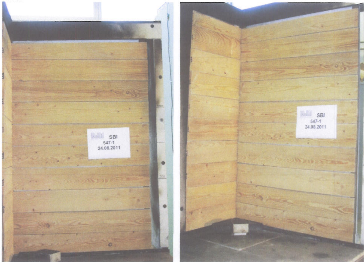
Fig. 1 Specimen mounting in SBI (Specimen No. 547-1).
